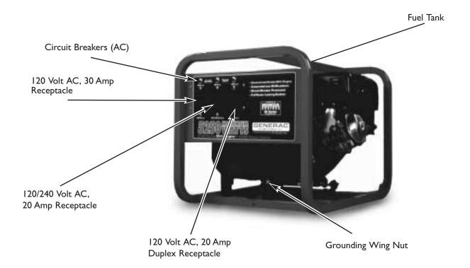
**I 20 Volt AC, 20 Amp Duplex Receptacle** — May be used to supply electrical power for the operation of I 20 Volt AC, 20 Amp, single phase, 60 Hz electrical lighting, appliance, tool and motor loads.
